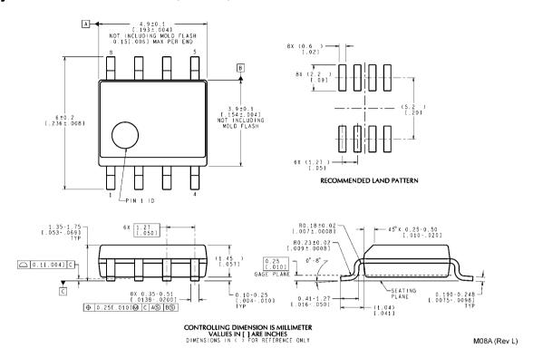
8-Lead (0.150 Wide) Molded Small Outline Package, JEDEC Order Number LM2671M-3.3, LM2671M-5.0, LM2671M-12 or LM2671M-ADJ NS Package Number M08A
